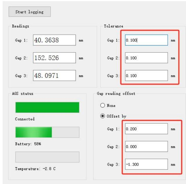
3. In the adjustment box for each gap, Enter the value you want the CGMS-software to display for the current measured gap .
