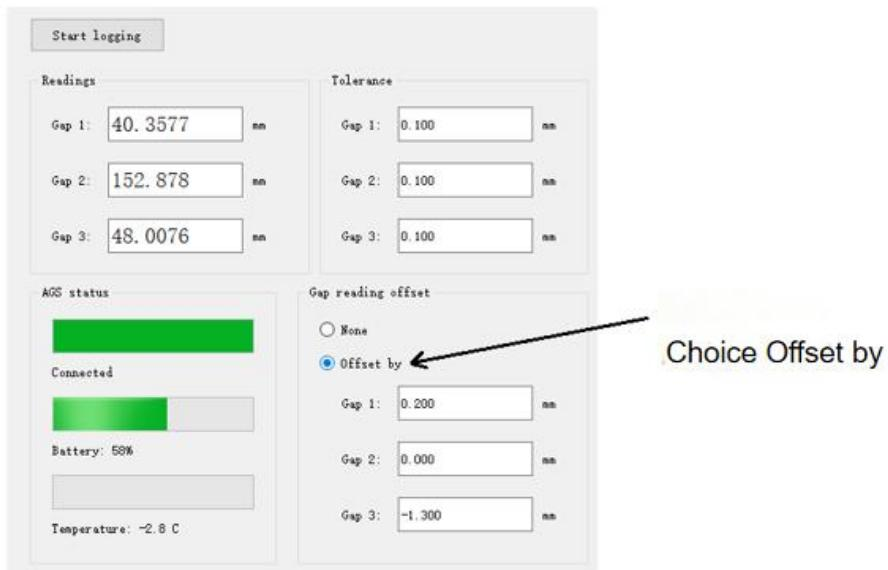
To stop CGMS-software from applying the gap offsets,in the Gap reading offset controls choose None .
